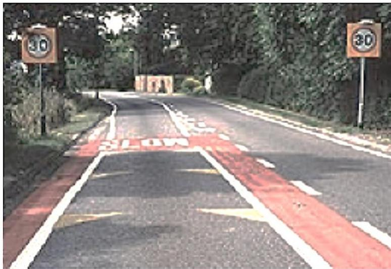
Figure 4: Example of ‘countdown’ approach to 30 mph speed limit
